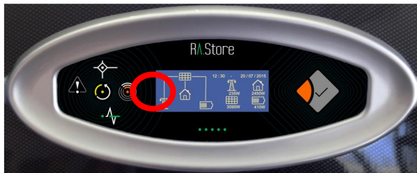
Picture 24 – Led light of communication switches on if the configuration has been done successfully
